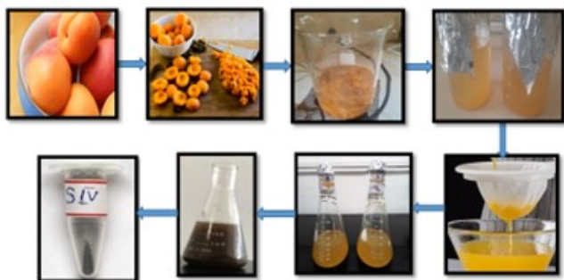
Figure 1: Schematic diagram for Green synthesis of AgNPs
